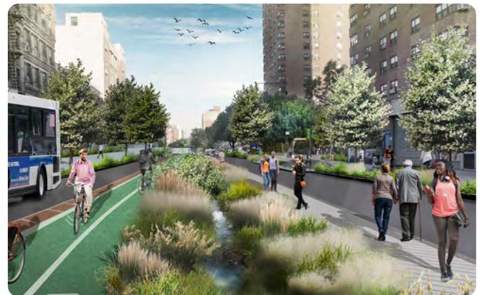
One of the team's proposed pilot projects to combat the bathtub effect in East Harlem was an integrated stormwater management/green infrastructure project along 106th Street paired with a reconfiguration of the right-of-way to better accommodate pedestrians, cyclists, and buses.
